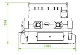
Operating Voltage – 400v. Frequency – 50hz. Connector plug fitted – 32amp three phase five pin. A+N+PE MCB (Minature circuit breaker) if fitted – Cat D
